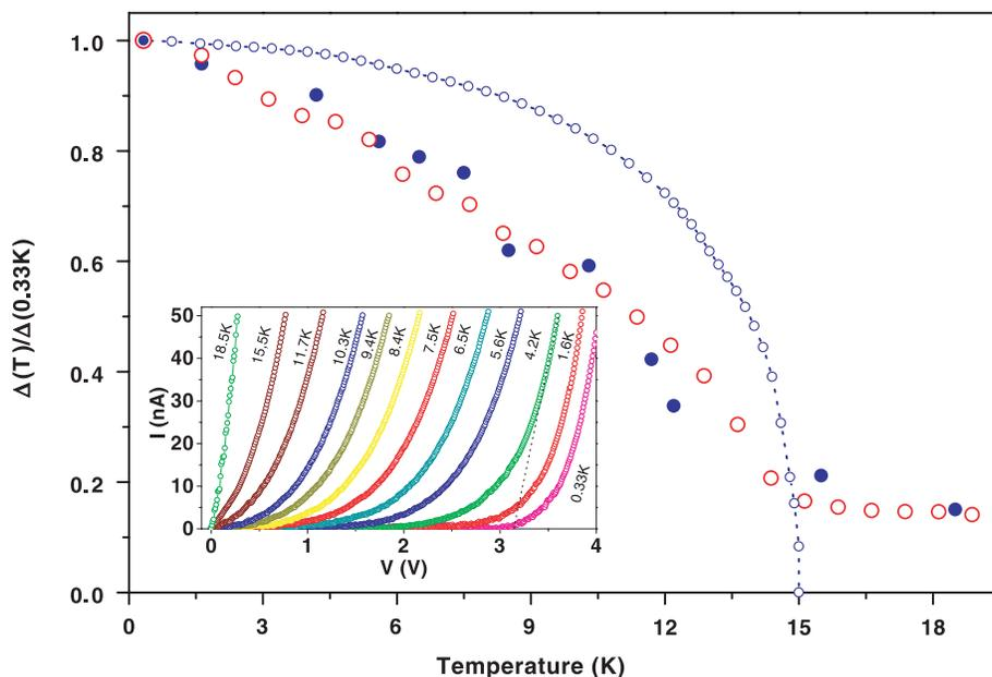
**Fig. 2.** Temperature dependence of the gap, normalized to its value at 0.33 K. Values shown are for theory (open symbols) and experiment (filled symbols).  $\circ$ - $\circ$  denotes the BCS gap. **(Inset)** The  $I$ - $V$  curves at various temperatures. The dashed line at 4.2 K illustrates the extrapolation from the high field. To a reasonable approximation, the intercept is proportional to the gap magnitude.
