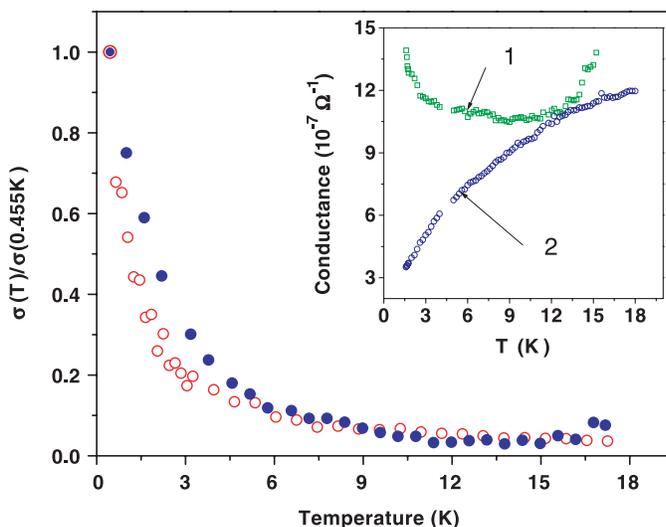
**Fig. 4.** The normalized conductivity plotted as a function of temperature for the thinnest part of the sample shown in Fig. 3,  $\sim 50$  nm thick. Experimental values (filled circles) and the theoretical predictions for the fluctuation supercurrent (open circles) are shown. The estimate for the lower bound of nanotube conductivity  $\sigma(0.445 \text{ K})$  is  $320 \text{ ohm}^{-1} \text{ cm}^{-1}$ . (Inset) The measured sample conductances, labeled as 1 and 2 in the text.
