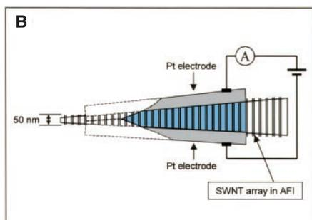
**Fig. 3.** (A) Scanning electron micrograph of the sample after thinning by argon milling. The dark region is a hole in the foil. Because the foil is translucent in its thinnest part, the bottom electrode is dimly visible. (B) A diagram of the sample. Shading indicates the part of the sample after the tip has been removed.
