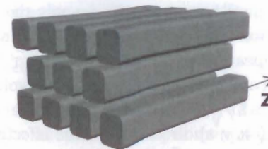
Figure 1.14 A cartoon picture of the model. The parallel nanowires form a 2D triangular lattice in x - y ( a - b ) plane. The nearest-neighbor nanowires interact with each other by weak Josephson coupling, denoted by the double-headed arrows. Adapted from Ref. [47].
